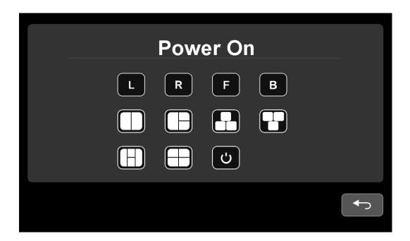
Power On menu option determines what video channels are displayed when the system first powers on.
