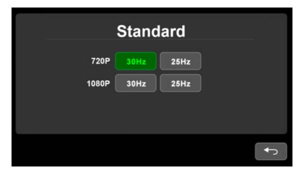
Standard setting interface (TV system setting in split-screen display mode), as shown in the Pic. above.
