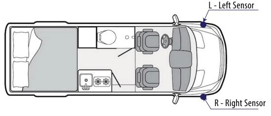
Step 2. Installation of the left/right turn trigger. Using the voltage Multi-meter, locate the left and right turn signal trigger wires behind the front turn signals. Once verified, connect the left and right signal wires of the RVS-130 wire harness to the correct signal wires.
