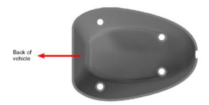
Why incorrect orientation is a problem: The microwave signal is emitted out of the larger end of the sensor. The sensor will sense objects coming toward it. So, if it is pointing in the wrong direction, it may sense things that are stationary, such as trees, as moving toward it. This is especially seen when the sensor is pointing toward the front of the vehicle (all stationary objects would be moving toward the sensor and cause false alarms).
