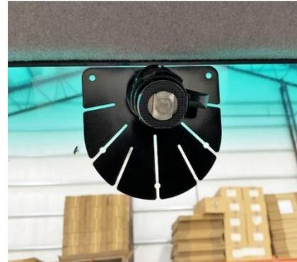
In most cases the RVS-MOUNT ("Fan" style w/double sided tape) will work best for the installation. It can be attached to the dash (with screws in addition to the 3M tape) or attached to the windshield using the 3M tape. **Note:** The windshield must be cleaned thoroughly with Isopropyl or denatured alcohol.
