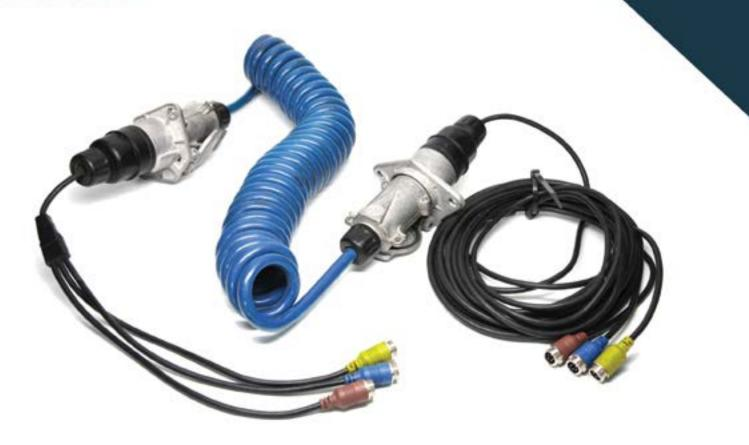
Commercial grade quick connect kit for multiple cameras. These cables allows one to wire his truck and trailer separately and connect/disconnect with just one pigtail cable. It comes with one mounting bracket for the back of the truck and one for the front of the trailer with a 12' pigtail that stretches between them.
